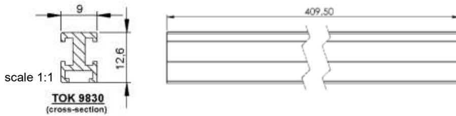
This BEAM is used to strengthen modules. It can be used in both the bottom module as well as the positioning module.
