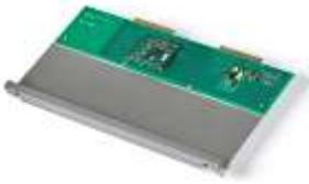
Boundary Scan Expansion Board developed in cooperation with JTAG.
