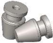
Peripheral positioning pins can be placed around the edges of the unit under test (UUT) to position the UUT on the positioning board. They are mainly used when insufficient space is available for a FAST-LOCK unit.
