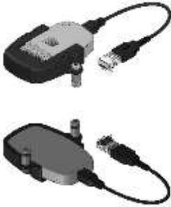
The ST-LINK V2 Holder is used to secure the ST-LINK V2 onto a module.
