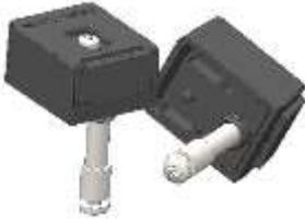
The TOK 9710 - FAST-LOCK is used to fixate the PCB during tests. FAST-LOCKS can be placed on all sides of the unit under test (UUT). It prevents tilting of the UUT by the force of the contacting probes. The screw on top of the FAST-LOCK allows for small adjustments of the FAST-LOCK's position on the positioning board. The pitch between each FAST-LOCK should be between 70 and 100mm.
