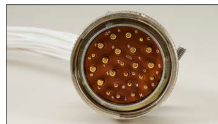
Connectors may contain several different size contacts.
