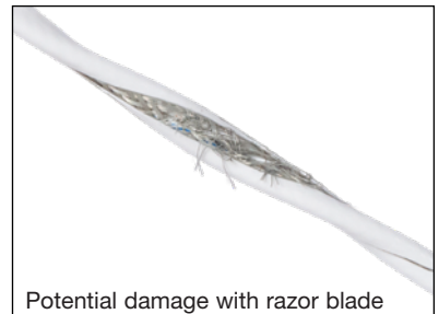
Potential damage with razor blade
