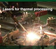
Lasers are used for many thermal processing tasks including resin welding, soldering, and hermetic sealing of glass as well as welding and quenching.
