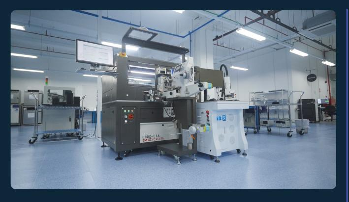
The Hi-Lo AT3-350B Automated Programming Systems can achieve up to 3000+ UPH and supports up to 64 sockets.
