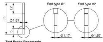
Test Probe Receptacle
