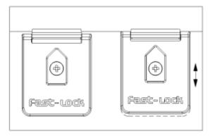
The FAST-LOCK can be adjusted horizontally after it has been placed on the module board. Loosen the screw on top of the FAST-LOCK to enable adjustment. The maximum adjustment is 0.2 mm forwards, and 0.3 mm backwards. Then fasten the screw to fix it in place. This is useful for ensuring a good fit with the UUT.
