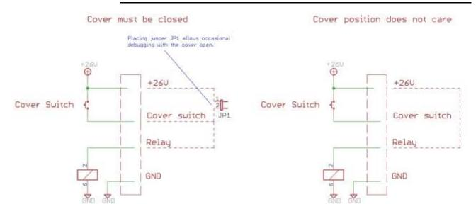
It is possible to add a relay on the TEST-OK module to control additional items. In this case, connect the relay between the 'Cover switch' and 'GND' pins.
