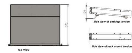
Width: 443 mm Depth: 372 mm Height: 62 mm
