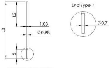
Test Probe Receptacle
