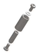
Adjustable peripheral positioning pins are adjustable (to a maximum of 0.8 mm per pin), allowing fine positioning of the UUT, after installation. There are two types available: the TOK 9771 - 8.8 (M3) and TOK 97 71 - 6 (M2).
