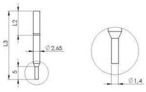
Test Probe Receptacle
