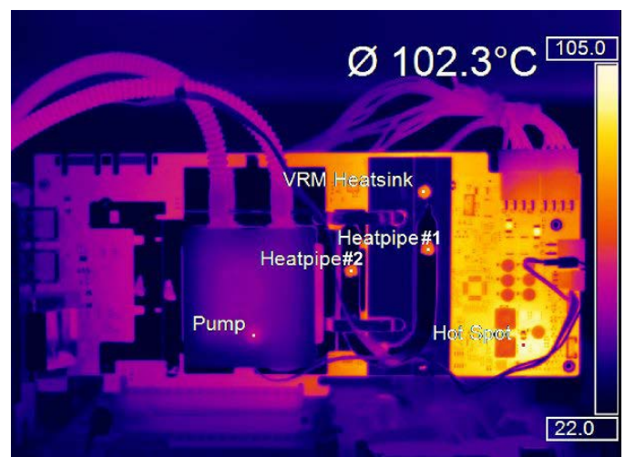
Thermal image of an operating motherboard Source: www.igorlab.de/en/ (Igor Wallossek)
