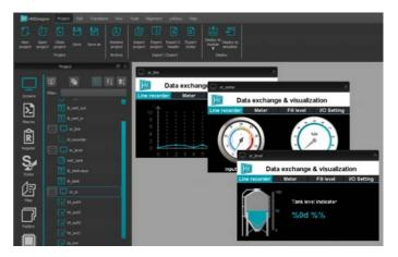
are possible without Modbus communication. The transfer of values, touch operations or the display of texts is carried out via freely definable Modbus registers. Floating point numbers can also be transmitted and displayed directly. Even multilingualism is supported.
