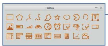
interfaces are created in no time at all. Objects are dragged and dropped into the virtual screen, where their size, angle of rotation and position can be easily adjusted with the mouse.
